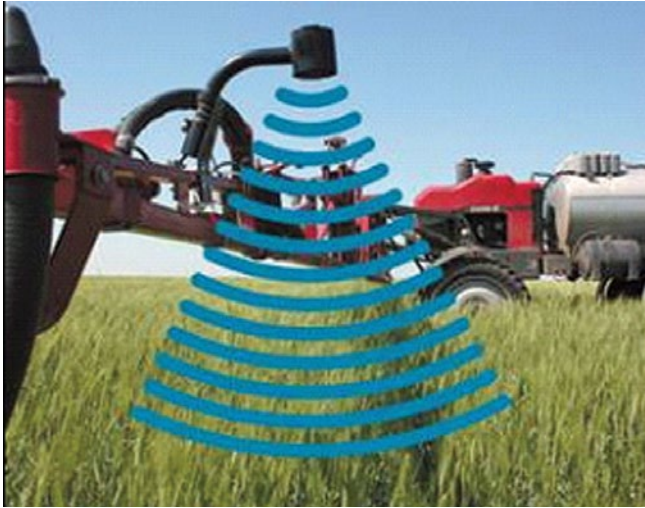
Figure 12. Spray-boom control to eliminate streaks and improper overlaps ( www.norac.ca/products.php ).
