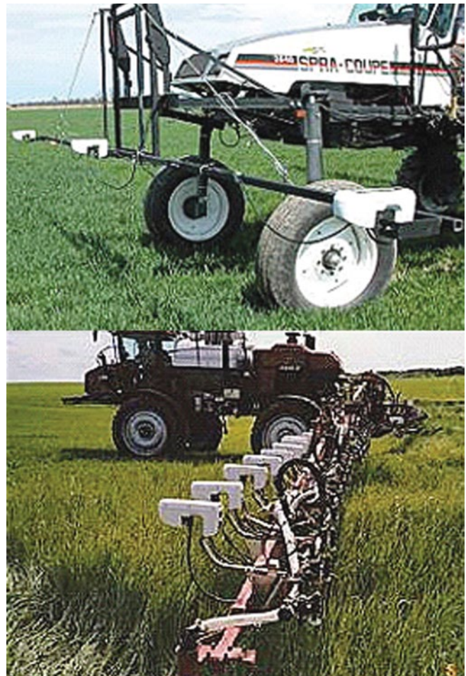
Figure 16. Optical sensor measuring Normalized Difference Vegetation Index (NDVI; GreenSeeker) and adjusting VRA nitrogen on wheat.
