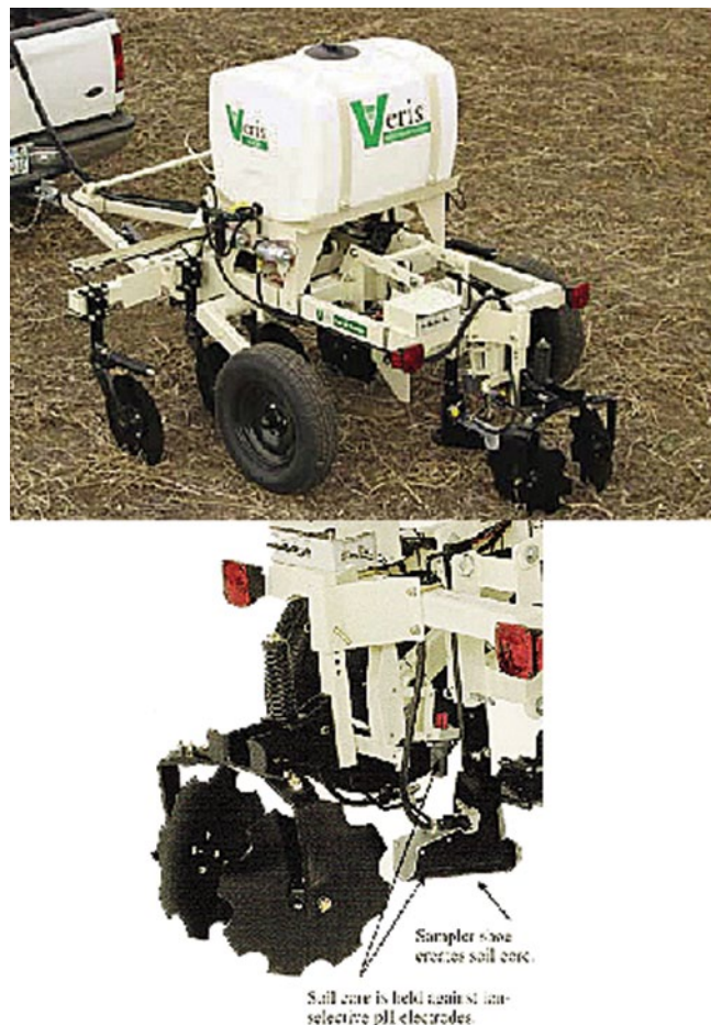
Figure 15. Veris Mobile Sensor Platform (MSP) equipped with “pH Manager” ( www.veristech.com/products/soilph.aspx ).
