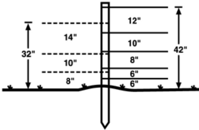
**Figure 1.** Appropriate spacing for three and five strand permanent and temporary electric fence.
